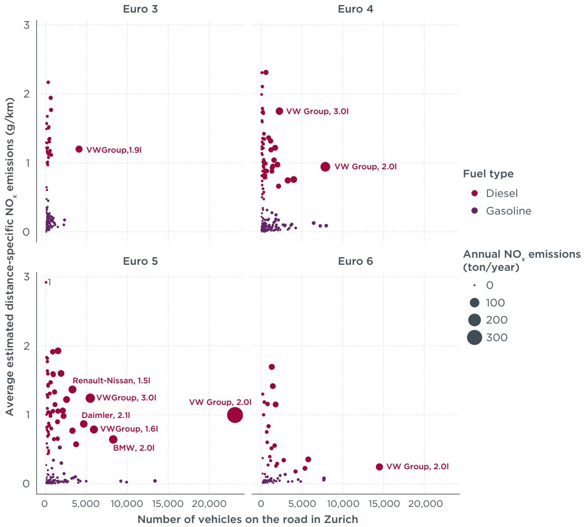
Figure 13. Mean distance-specific NO x emissions and number of registered vehicles in Zurich. Each marker represents a vehicle family. Annual NO x emissions of each vehicle family estimated using average vehicle mileage data. Top 10 vehicle families in terms of estimated annual NO x emissions across all Euro standards are labeled in the chart.
